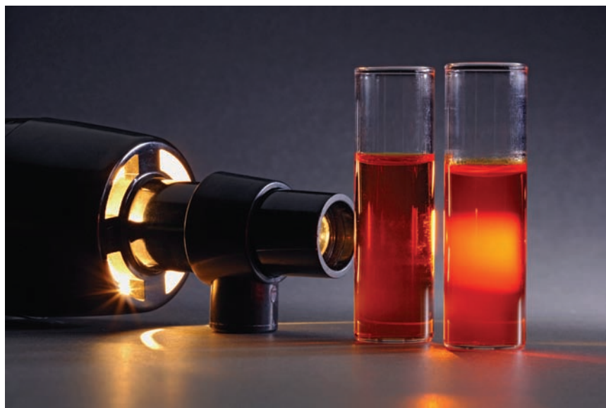
▲ Figure 13.25 Tyndall effect in the laboratory. The glass on the right contains a colloidal dispersion; that on the left contains a solution.
