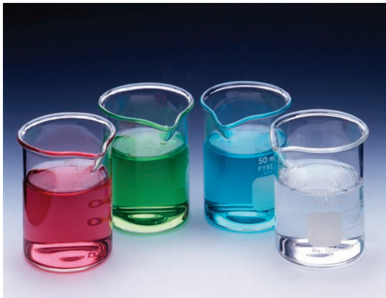
▲ Figure 23.4 Aqueous solutions of transition metal ions. Left to right: \text{Co}^{2+} , \text{Ni}^{2+} , \text{Cu}^{2+} , and \text{Zn}^{2+} . The counterion is nitrate in all cases.
