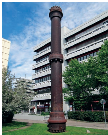
▲ Figure 15.4 A high-pressure steel reactor used in the Haber process is on display at Karlsruhe Institute of Technology in Germany where the Haber process was developed.
