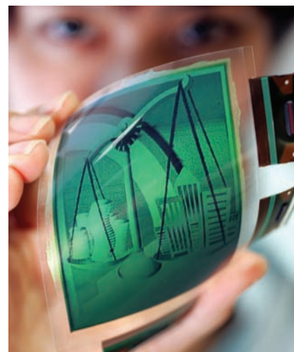
▲ Figure 11.34 Electronic paper (e-paper) based on cholesteric liquid crystal technology. Electronic paper mimics the appearance of ordinary ink on paper (like a page of a book or magazine). It has numerous potential uses including thin displays on walls, electronic labels, and electronic book readers.
