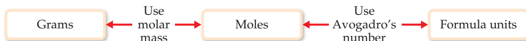
▲ Figure 3.12 Procedure for interconverting mass and number of formula units. The number of moles of the substance is central to the calculation. Thus, the mole concept can be thought of as the bridge between the mass of a sample in grams and the number of formula units contained in the sample.
