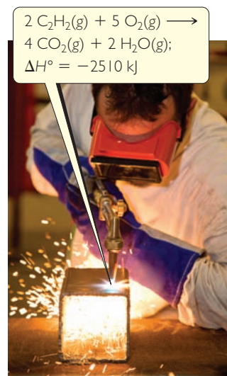
▲ Figure 22.12 Welding with an oxyacetylene torch.
