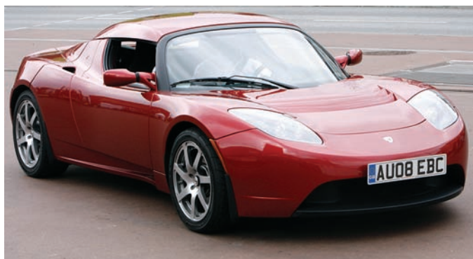
▲ Figure 20.22 Electric automobile. The Tesla Roadster is a fully electric vehicle powered by Li-ion batteries that can go over 200 miles per charge.
