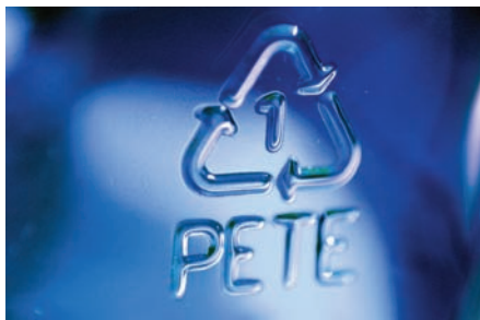
► Figure 12.36 Recycling symbols. Most plastic containers manufactured today carry a recycling symbol indicating the type of polymer used to make the container and the polymer's suitability for recycling.
