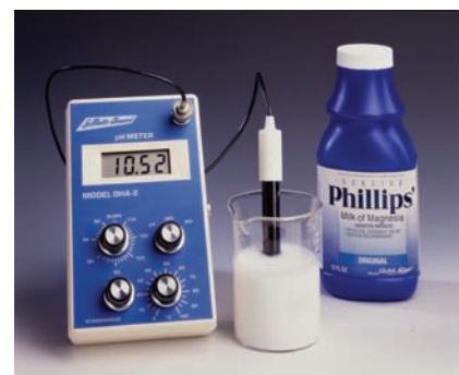
▲ Figure 16.7 A digital pH meter. The device is a millivoltmeter, and the electrodes immersed in a solution produce a voltage that depends on the pH of the solution.
