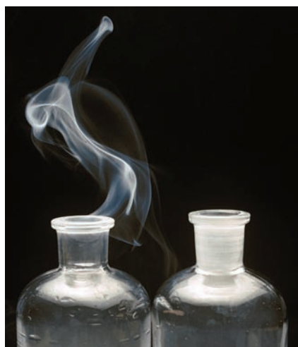
▲ Figure 16.3 Fog of NH 4 Cl(s) caused by the reaction of HCl(g) and NH 3 (g).
