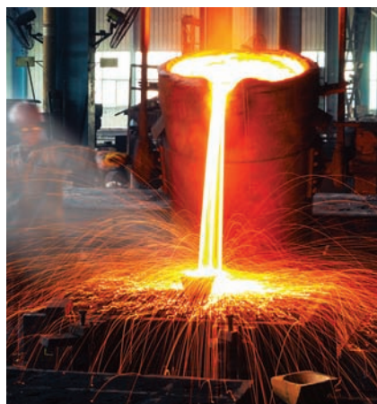
▲ Figure 6.5 Color and temperature. The color and intensity of the light emitted by a hot object, such as this pour of molten steel, depend on the temperature of the object.
