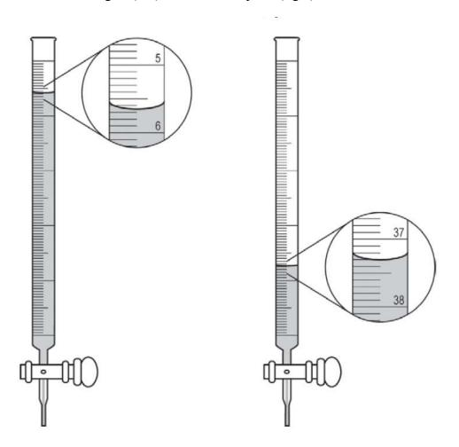
(a) In the table below. record the initial and final buret readings and the calculated value for the volume of 0.665 M NaOH(aq) required to reach the end point.
